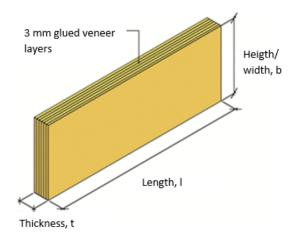
Fig. 1 Stora Enso LVL. In S-grade and T-grade all veneers has the fiber direction running parallel to the longitudinal direction. In X-grade the veneers are regularly placed crosswise and parallel to the beam's longitudinal direction
